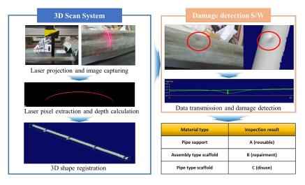
Fig. 1 Procedure of the proposed inspection scheme
